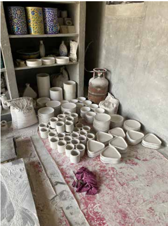
The pieces are removed from mould and kept aside for drying before hand painting the actual blue pottery motifs. Picture Courtesy: Nayan Menghani
