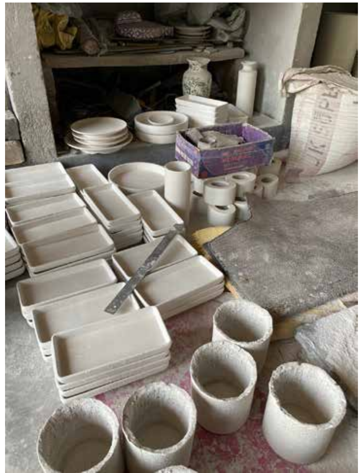
The pieces are removed from mould and kept aside for drying before hand painting the actual blue pottery motifs. Picture Courtesy: Nayan Menghani
